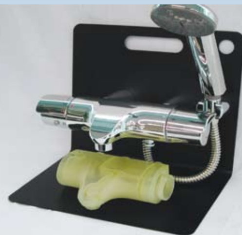
Model before the plating process (photograph – bottom) and model after the plating process (photograph – top)
